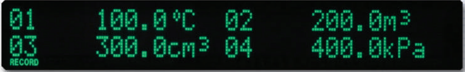
Two groups are alternately displayed: 18 dot model 1Gr (1 to 12ch), 2Gr (13 to 18ch) 24 dot model 1Gr (1 to 12ch), 2Gr (13 to 24ch)
