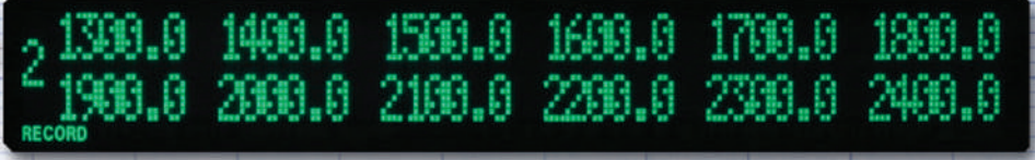
Two groups are alternately displayed: 18 dot model 1Gr (1 to 12ch), 2Gr (13 to 18ch) 24 dot model 1Gr (1 to 12ch), 2Gr (13 to 24ch)
